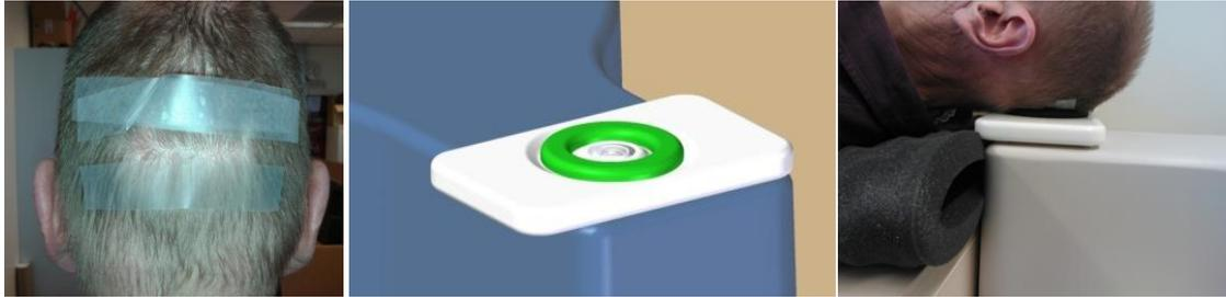
Ergonomic detachable support for underarm measurements (support is fixed to the analyzer)
